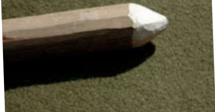
The end that fits the hand hold device - sharpened to minimise friction
